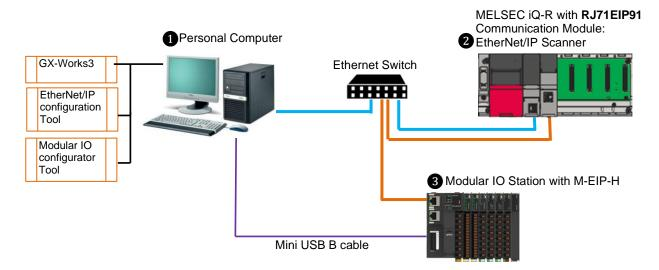
Modular IO station supports 2 Ethernet ports (ETH1 and ETH2; Layer 2 switch with DLR support). But scanner RJ1EIP91 supports 1 Ethernet port. User can connect any one port of Modular IO station to Ethernet/IP network.
